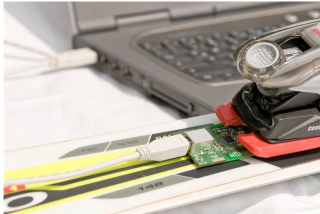
Figure 1: NFC-Hardware used for the protection of a ski.
